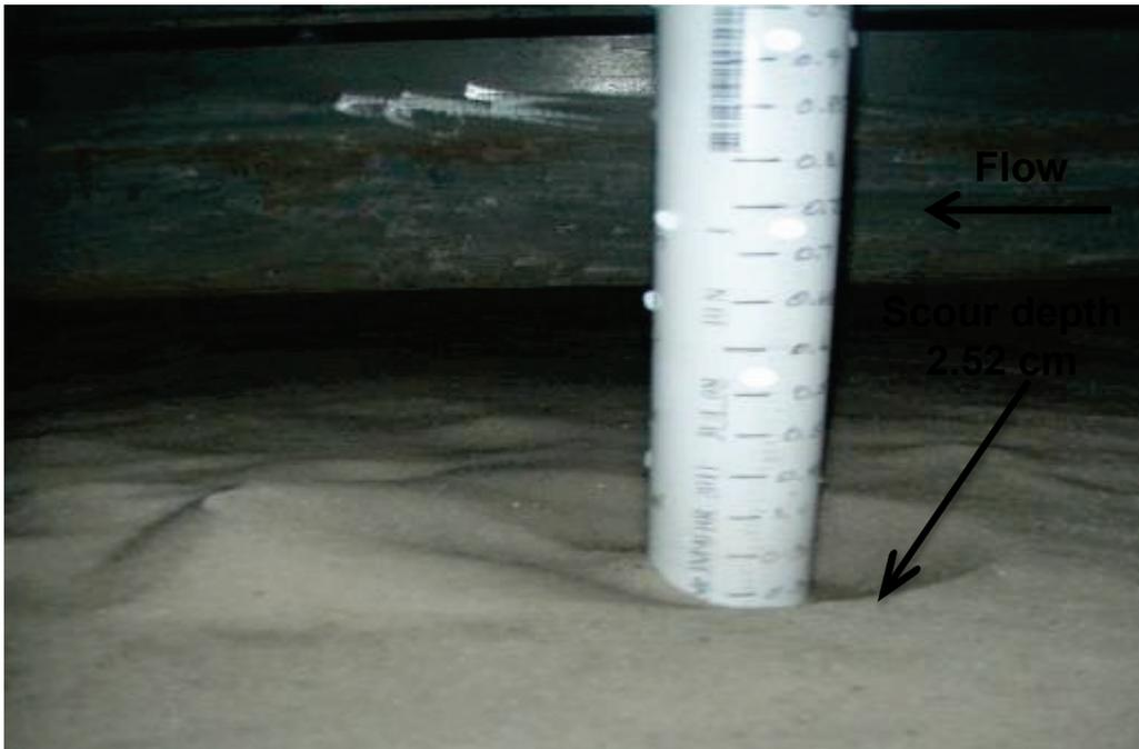
Figure A-11. Test 4. Scour upstream of 4.76-cm cylindrical obstruction, full flow depth obstruction,  $Q=0.02 \text{ m}^3/\text{s}$ ,  $V_{\text{avg}}=21.31 \text{ cm/s}$ , flow depth = 7.62 cm,  $t = 3 \text{ hr}$ .
