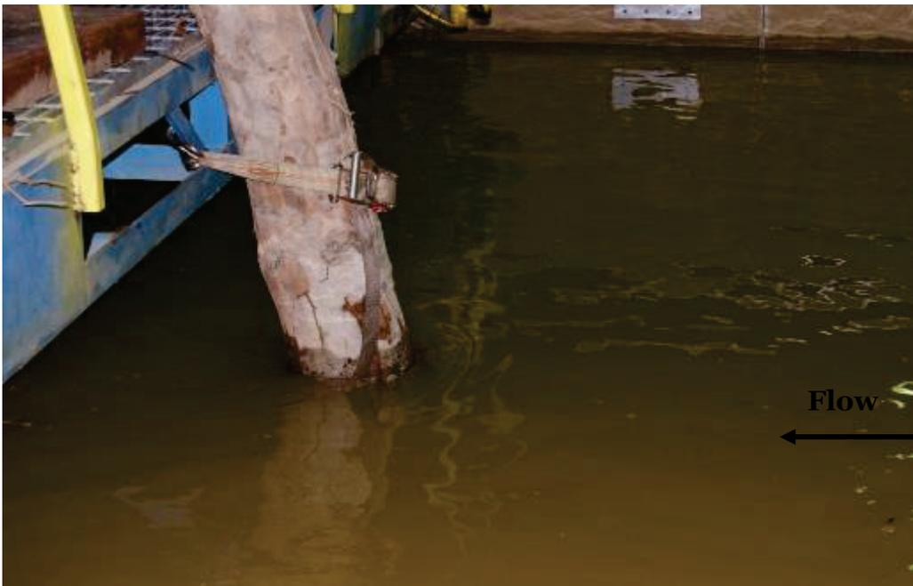
The model flume was gradually drained and photographs for photogrammetry analysis were recorded. The results of the photogrammetry point cloud and analysis software for Test 10B are shown below in Figures B-29 and B-30. Test 10B produced a scour hole approximately 17.1 cm deep on the right side of the tree looking downstream.
