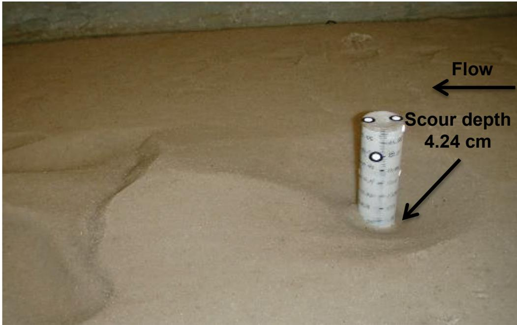
Figure A-13. Test 6. Scour upstream of 4.76-cm cylindrical obstruction, obstruction submerged 7.62 cm (50 percent flow depth obstruction),  $Q=0.04 \text{ m}^3/\text{s}$ ,  $V_{\text{avg}}=27.43 \text{ cm/s}$ , flow depth = 15.24 cm,  $t = 3 \text{ hr}$ .
