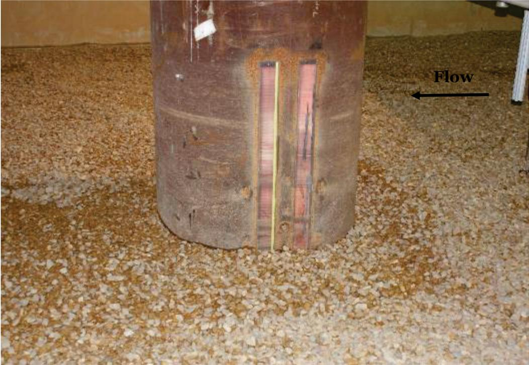
Figure B-9. Pretest photogrammetry point cloud of 0.92-m-diam cylinder.
