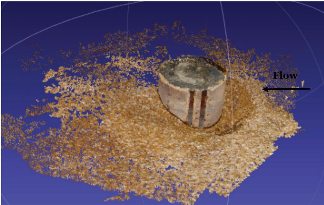
Figure B-17. Analysis of Test 4B using Crater Pro® Software, 0.92-m-diam cylinder in gravel, submerged flow,  $V_{avg} = 0.76$  m/s,  $d = 0.7$  m,  $t = 7.5$  hr.
