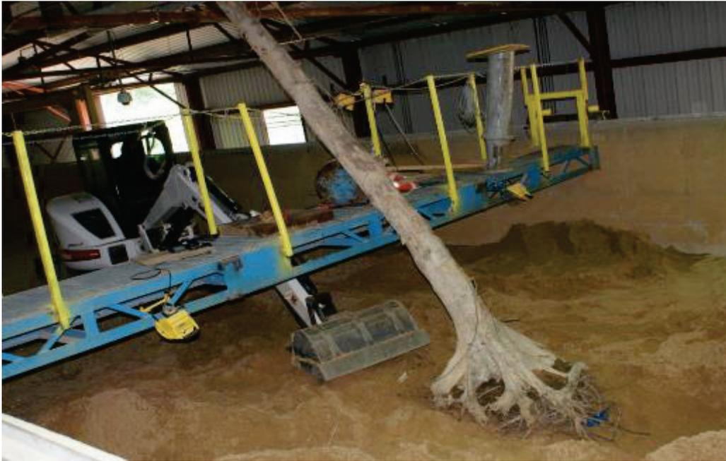
Figure B-27. Test 9B, tree in vertical position in sand, fully obstructed flow,  $V_{avg} = 0.35$  m/s,  $d = 0.7$  m,  $t = 3$  hr.
