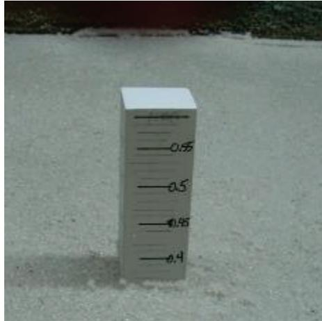
Figure A-19b. Test 7.  $Q=0.04$  m<sup>3</sup>/s,  $V_{avg}=27.43$  cm/s, flow depth = 15.24 cm,  $t = 3$  hr.
