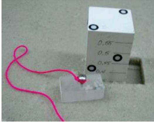
Figure A-28b. Test 14.  $Q=0.04$  m<sup>3</sup>/s,  $V_{avg}=27.43$  cm/s, flow depth = 15.24 cm,  $t = 3$  hr.
