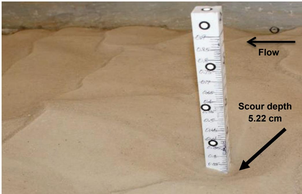
Figure A-38. Test 26. Scour upstream of 5.08-cm-square obstruction, 100 percent flow depth obstruction,  $Q=0.04 \text{ m}^3/\text{s}$ ,  $V_{\text{avg}} = 27.43 \text{ cm/s}$ , flow depth = 15.24 cm,  $t = 3 \text{ hr}$ .
