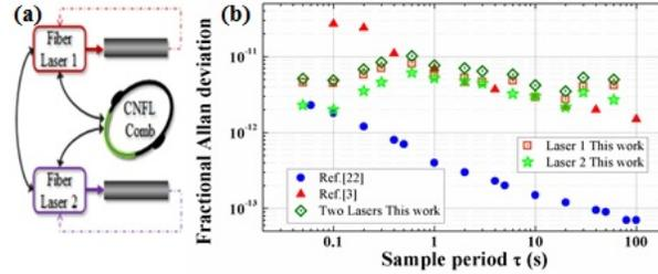
Fig. 9. (a) Schematic of the three-cornered hat measurement between two acetylene-stabilized fiber lasers and a phase stabilized CNFL comb. (b) Fractional Allan deviation of beat frequency between two acetylene-stabilized fiber lasers, compared with Ref. [51] and Ref. [34]. The individual stability of each laser obtained from three-cornered hat measurement is also shown.
