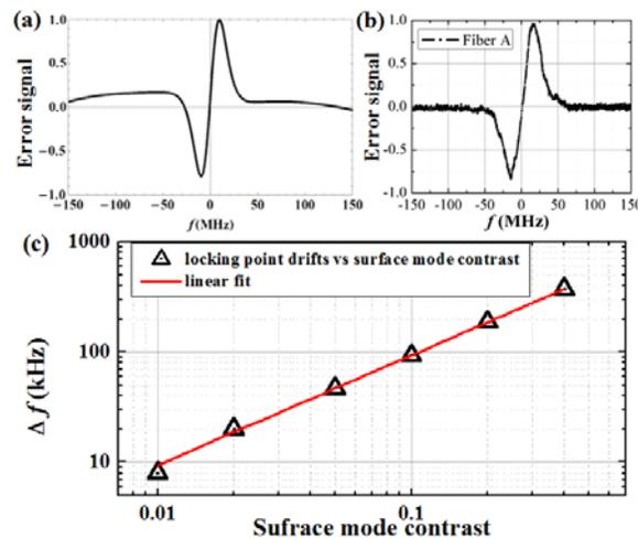
Fig. 14. (a) Calculated error signal in acetylene-filled 10  $\mu\text{m}$  PBGF with the nonlinear effect caused by pump power modulation; (b) experimental error signal; (c) Calculated maximum locking frequency change versus different surface mode contrast when varying only  $\Delta\Phi$  (not  $\Delta\Phi_{NL}$ ) by  $\pi$  to mimic slow thermal drift.
