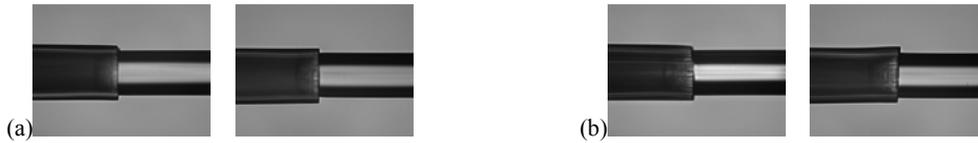
Fig. 20: side-views of (a) a conventional splice and (b) an angle splice of PRISM fiber and SMF-28.
