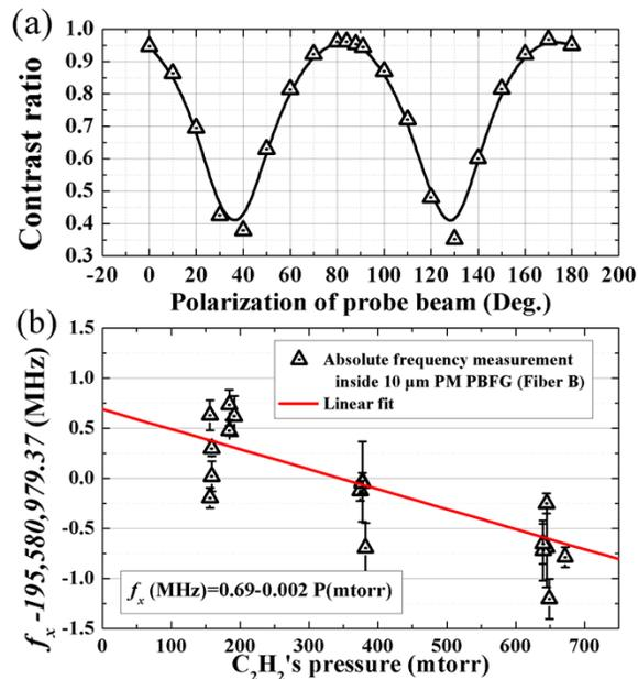
Fig. 15 (a) Contrast ratio of probe power exiting fiber vs. the angle of probe polarization in vacuum, solid line fitting curve of measured data, (b) Absolute frequency measurement of  $^{12}C_2H_2$  P(13) line inside 10  $\mu$ m PM PBGF (Fiber B); zero frequency corresponds to the published value [44].
