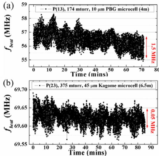
Fig. 16 (a) Beat frequency vs. time in  $^{12}\text{C}_2\text{H}_2$ -filled  $10 \mu\text{m}$  PBGF PMC for the P(13) line transition, (b) beat frequency vs. time in  $^{12}\text{C}_2\text{H}_2$ -filled  $45 \mu\text{m}$  kagome PMC for the P(23) line transition.
