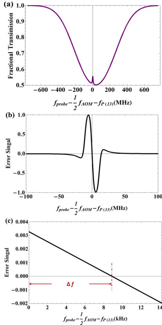
Fig. 10 (a) The calculated SAS of P(13) line of  $^{12}\text{C}_2\text{H}_2$ , with a FT of 50%, and exiting fiber pump power of 32 mW; (b) the normalized dispersive error signal of the P(13) line. The calculated error signal is proportional to what is detected by the PD; (c) same as (b) but plotted over smaller range to show the frequency of the zero-crossing.
