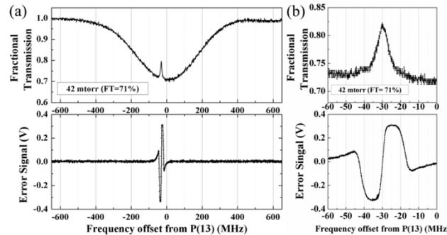
Fig. 8. (a) top: Fractional transmission of a 4.1 m long kagome HC-PCF with a  $^{12}\text{C}_2\text{H}_2$  pressure of 42 mtorr, and a pump power of 25 mW exiting the fiber, bottom: error signal of sub-Doppler versus scanned frequency away from the P(13) transition. The laser frequency was scanned at 1.2 GHz/sec. (b) same as (a), but zoomed in on the sub-Doppler absorption feature.
