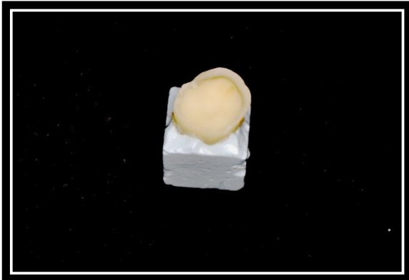
C- Mounted after diamond saw cut
