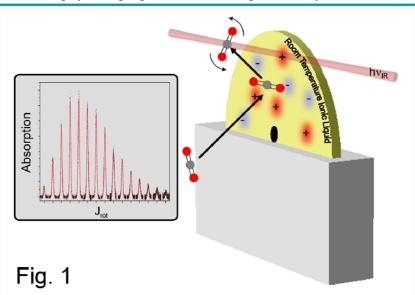
from such hyperthermal surface scattering events have been monitored by high resolution diode laser absorption spectroscopy as a function of i) cation alkyl chain length and ii) anion size, and analyzed to yield the propensity for trapping-desorption (TD) vs. impulsive scattering (IS)
