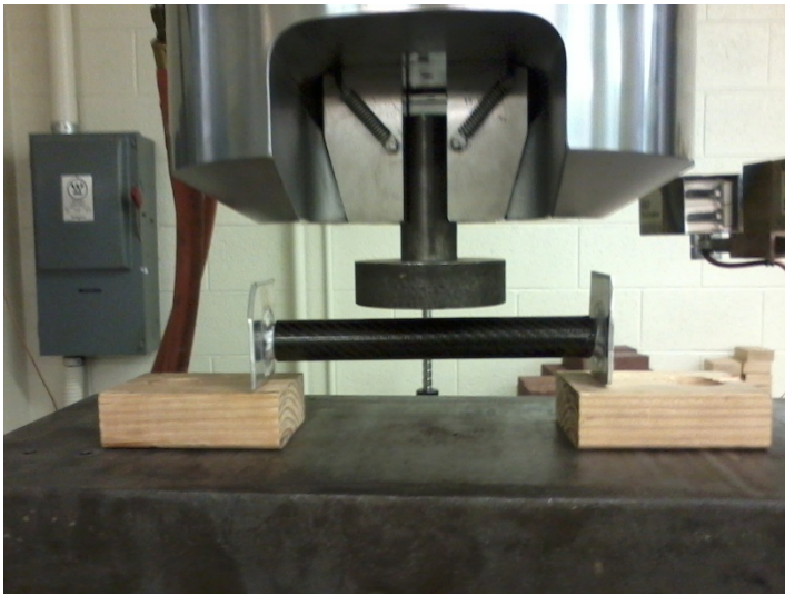
Figure 7: The testing method used to ensure the welds were sufficiently strong.
