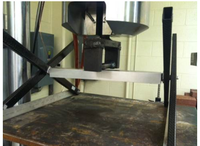
Figure 4: Load test done on structural beams.
