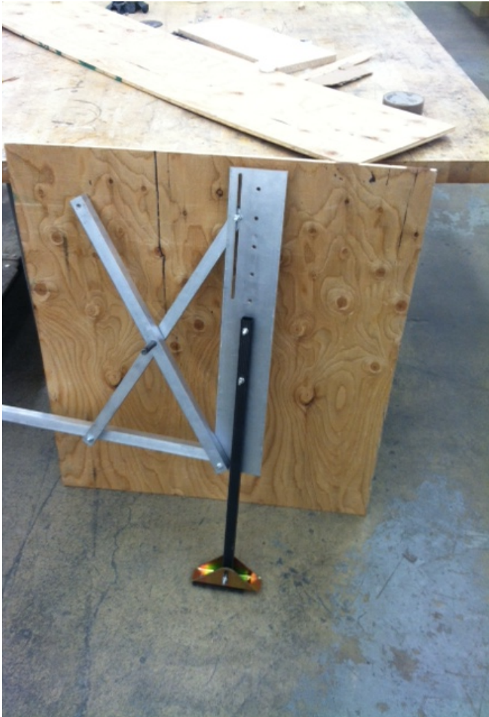
Prototype of attachment that could be used to adjust the bridge so as to be used on uneven surfaces.
