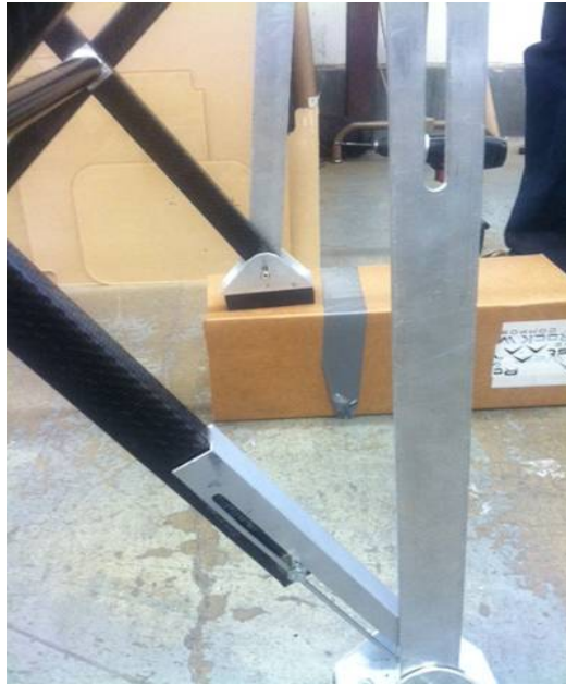
Figure 10: The attachment can be adjusted to lengthen one side of the bridge, enabling it to be used on uneven surfaces.
