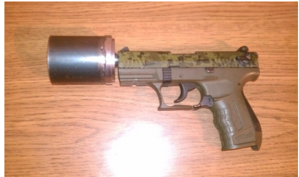
Figure 12 –Golf ball launcher attached to a .22lr handgun
