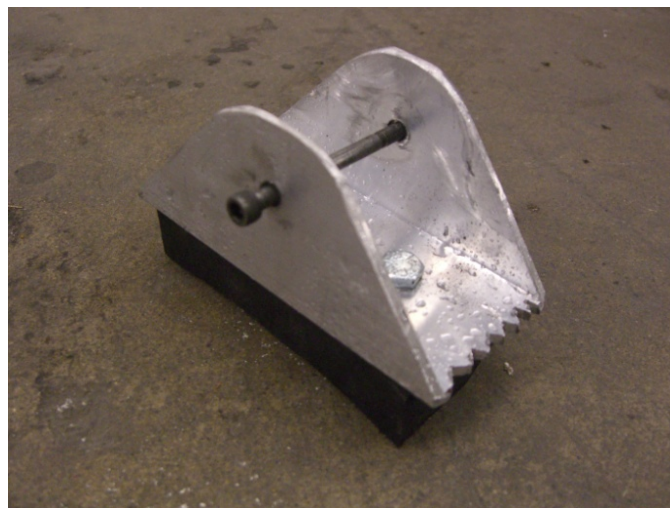
Figure 9: The foot of the bridge is designed to grip both hard and soft surfaces.
