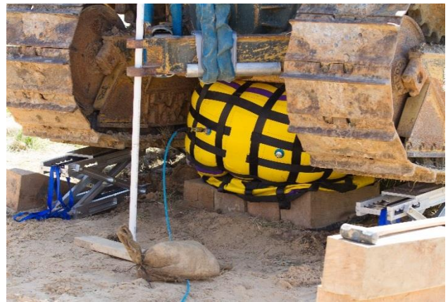
Figure 7: Heavy Lift Kit Implementation on D6 Bulldozer
