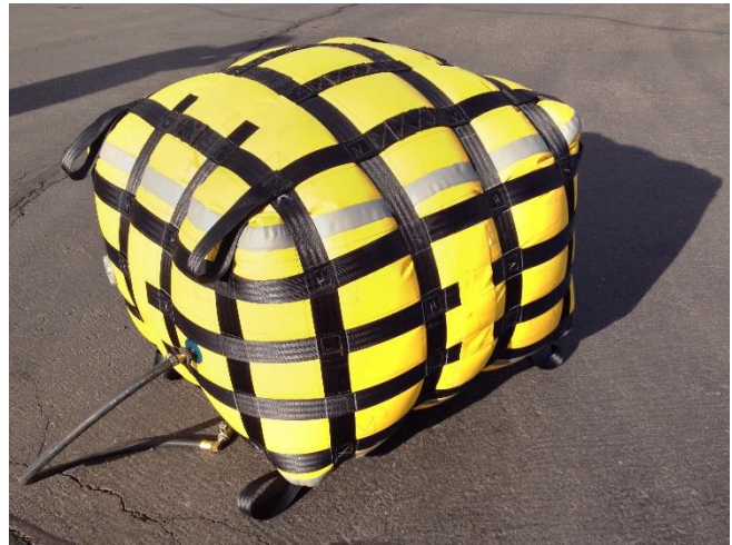
Figure 2: Completed Airbag capable of lifting 25,000 lbs
