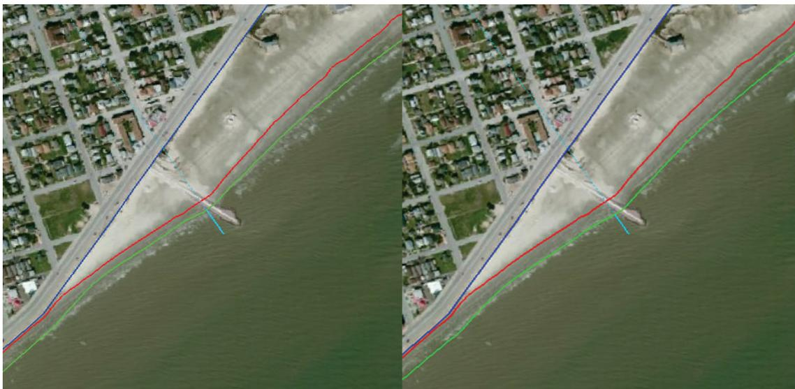
Although the structural alternatives result in slightly different calculated shorelines than the no-action alternative, none of the structural alternatives independently resulted in shoreline advance along the seawall; therefore, modifying the structures as a part of the sand management strategy is not recommended. Some of the structural alternatives were modeled in conjunction with beach fills, and those alternatives are presented later in this chapter.
