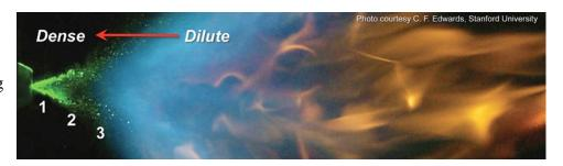
heating and evaporation occur within 1 ms of fuel leaving the fuel injector. This atomization proves is often the limiting process in combustion, which occurs only in the gas phase.
