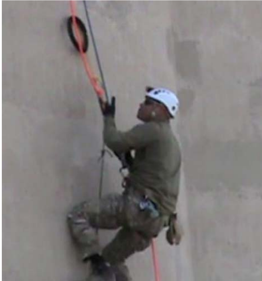
Fig. 7 A pararescue jumper tests the frayed rope adhesive bond by putting his whole weight on it, at the competition in Ohio in April 2012.
