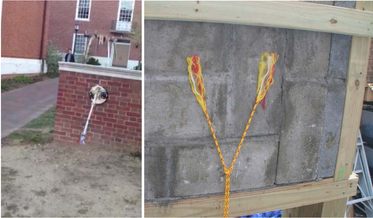
Fig. 6 Left: the vacuum cup and its boom detach from the quadcopter and remain attached to the wall by suction from two ducted fans in the assembly. The epoxy adhesive cured within about 5 minutes. Right: the frayed rope bonded to a test wall.
