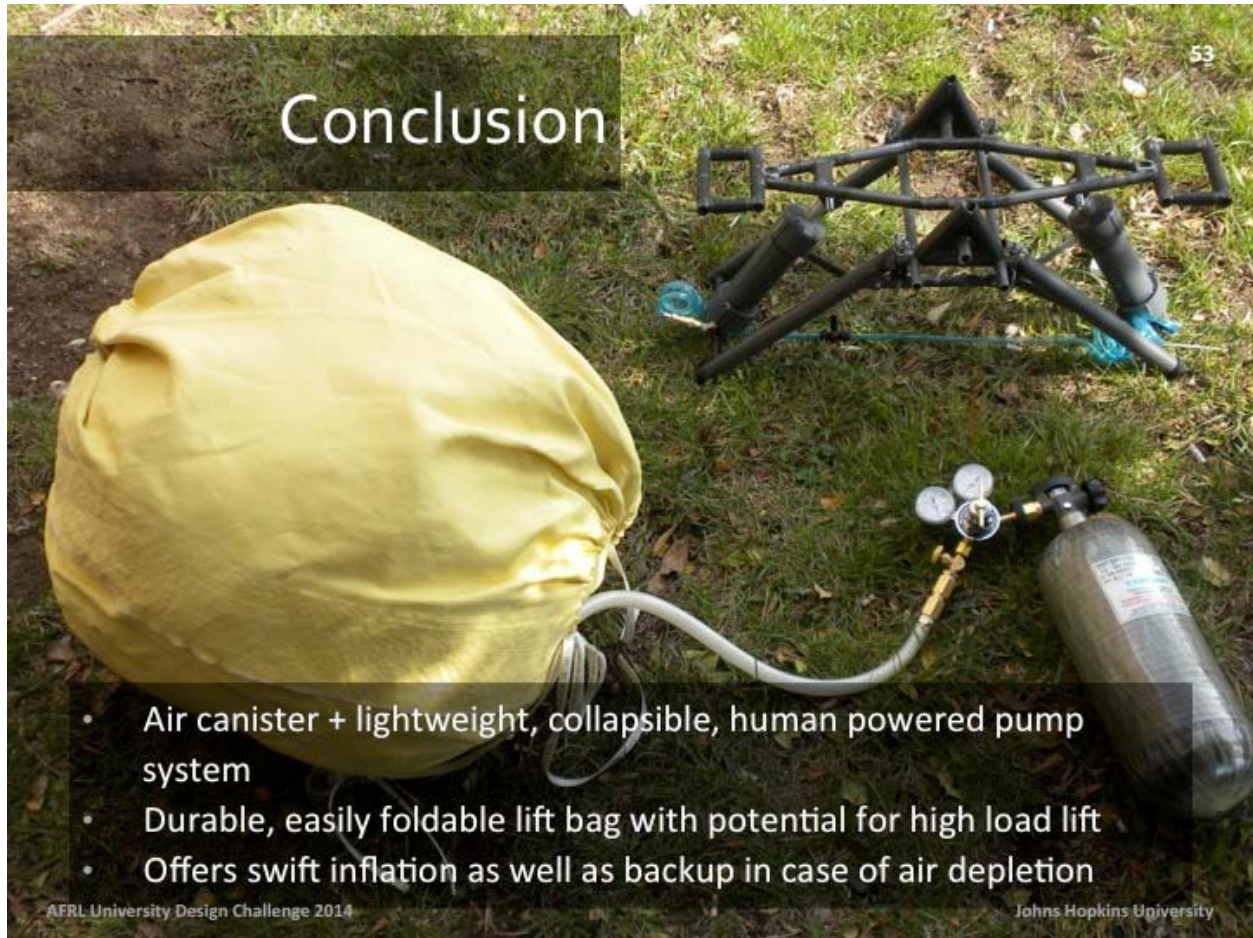
Fig. 10 Team AFRL air bag, custom pump and commercial SCUBA cylinder.
