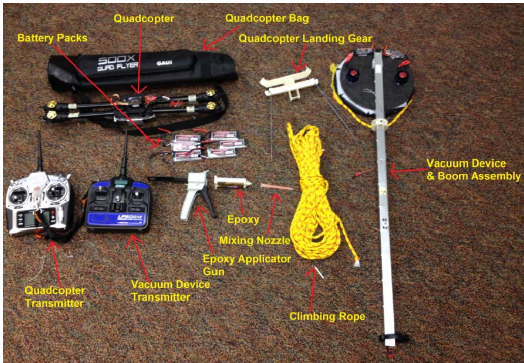
Fig. 2 All parts of SCALE system unloaded from the rucksack.
