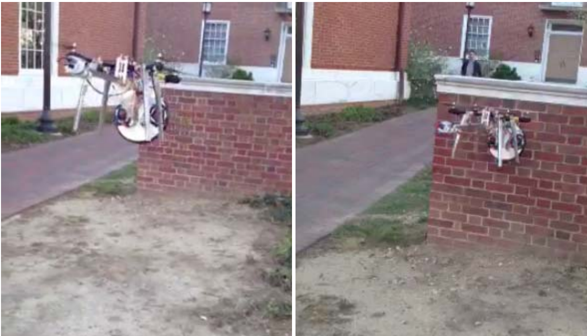
Fig. 5 The quadcopter, carrying the vacuum cup, is then flown to the attachment site and presses the vacuum cup to the wall.
