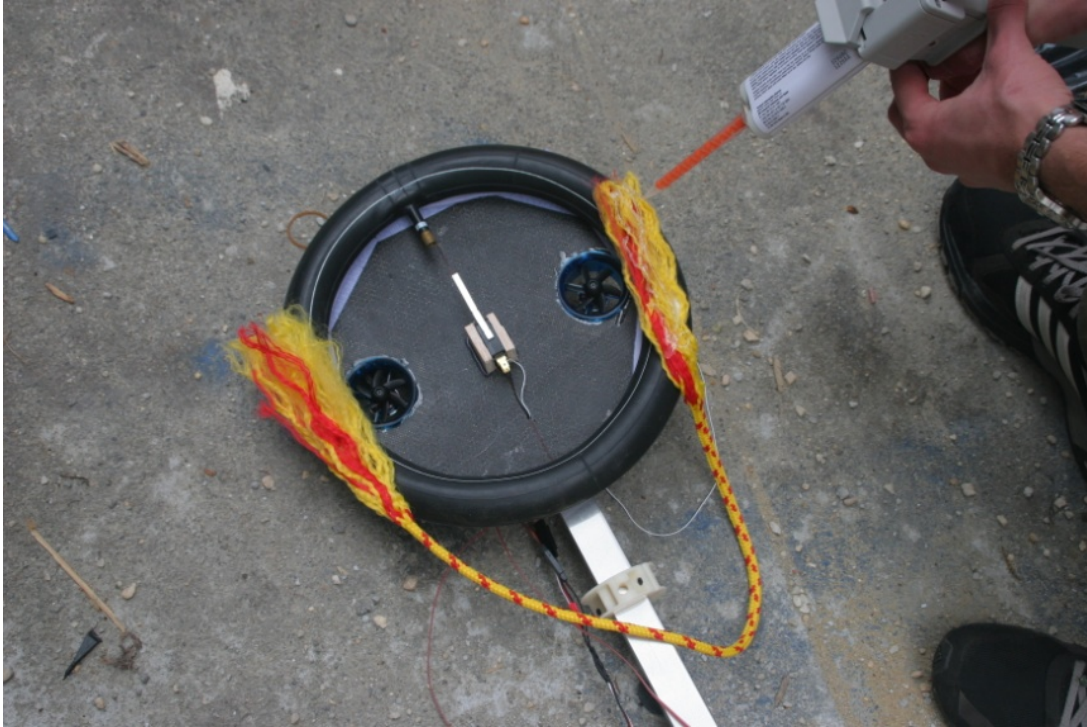
Fig. 4 Showing epoxy application to the frayed rope attachment on the vacuum cup.
