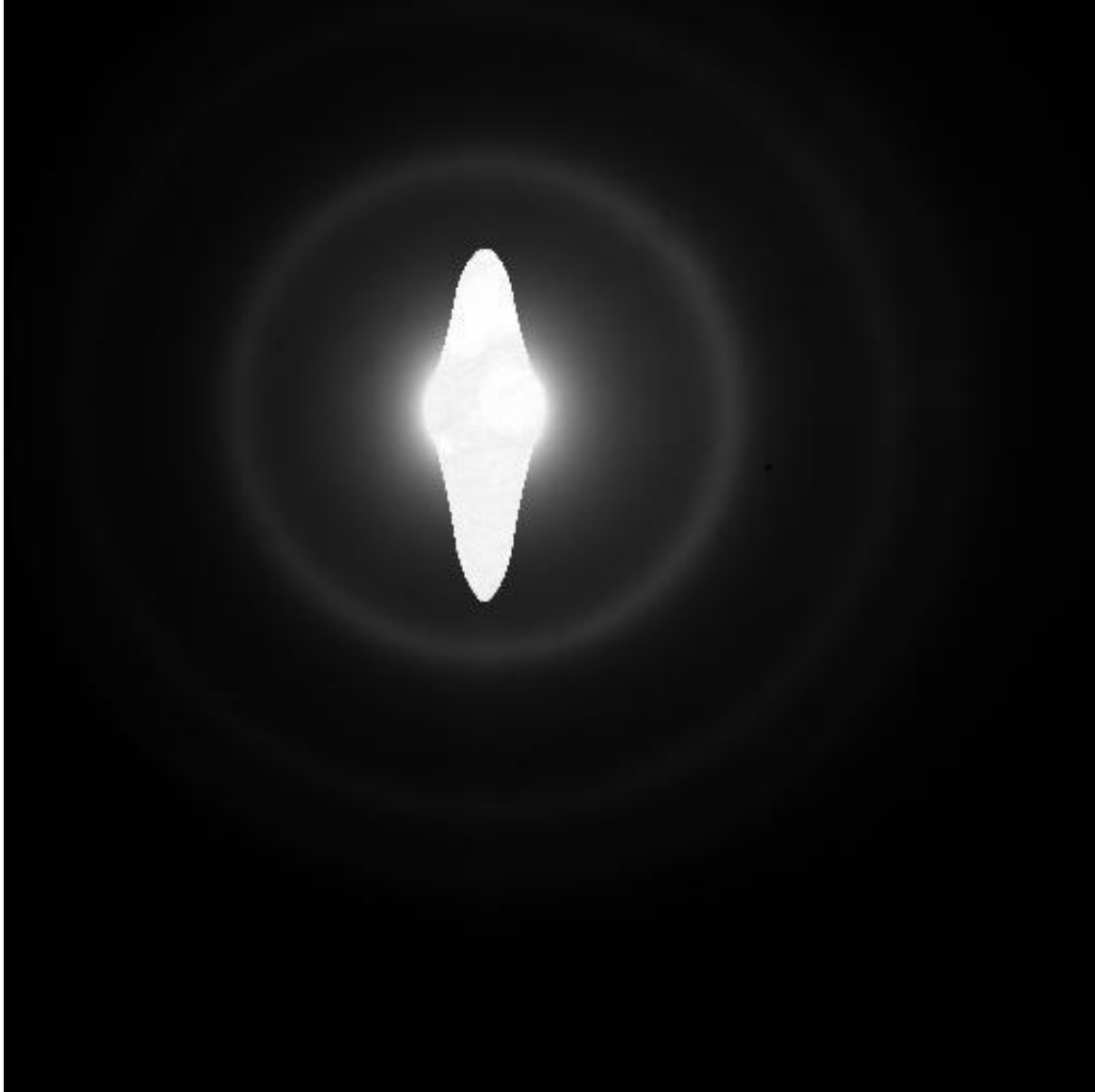
Figure 4 Selected area electron diffraction pattern showing broad rings consisting of very faint hidden sharp rings
