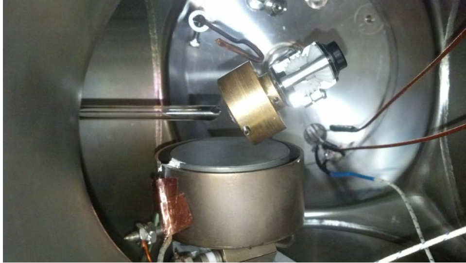
Figure 4.2 Image of the PPD chamber showing the rotating target holder, quartz nozzle, and substrate heater.
