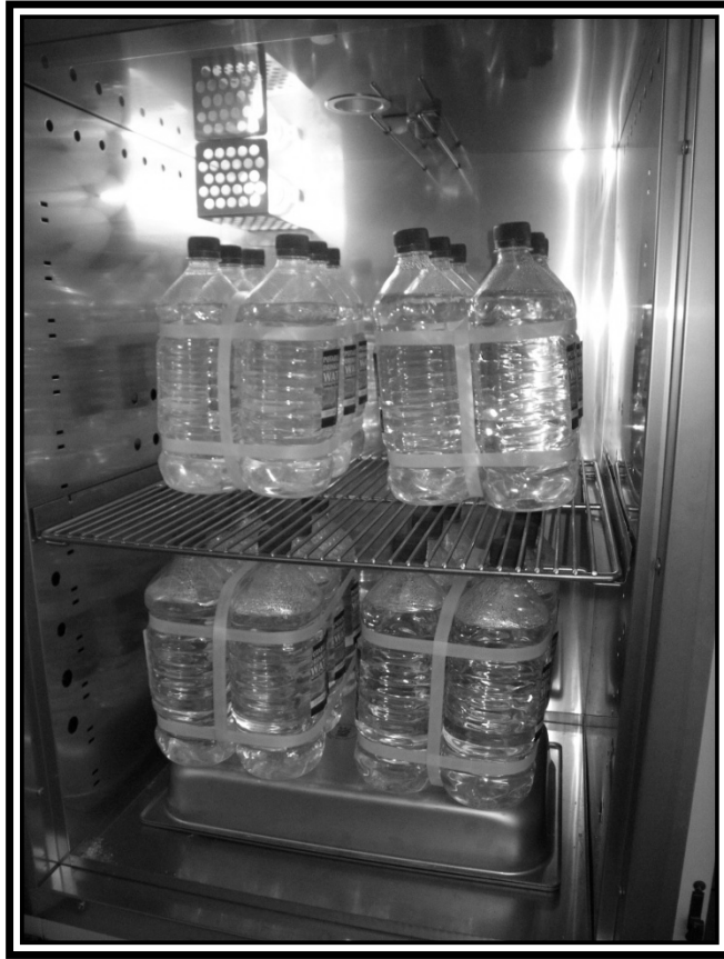
Figure 5: EWPS Water Bottles inside 60°C Laboratory Oven
