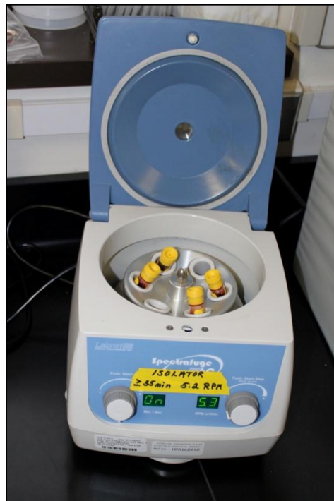
Figure 17: Centrifugation of Isolator™ 10 tubes
