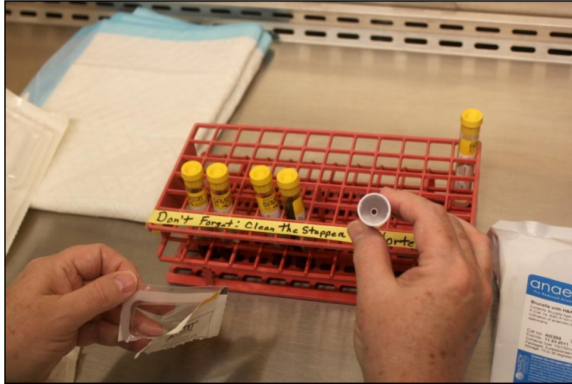
Figure 19: Placement of Isostat ® cap on Isolator ™ 10 tubes using Isostat ® press
