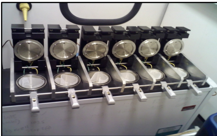
Figure 4. As shown, a Markes \mu -CTE with (n=6) 45 ml stainless steel cups. DDT treated polyester netting (3cm x 15cm) placed inside each stainless steel cup.
