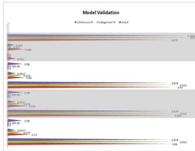
Figure 6: Comparison of prediction results for four sol-gel samples shown in Table 1 – red is Actual, Green is Categorical and Purple is Continuous fit.
