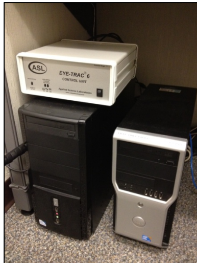
Picture 2: ASL EYE-TRAC 6 Control Unit, Control Computer, and Stimulus Computer
