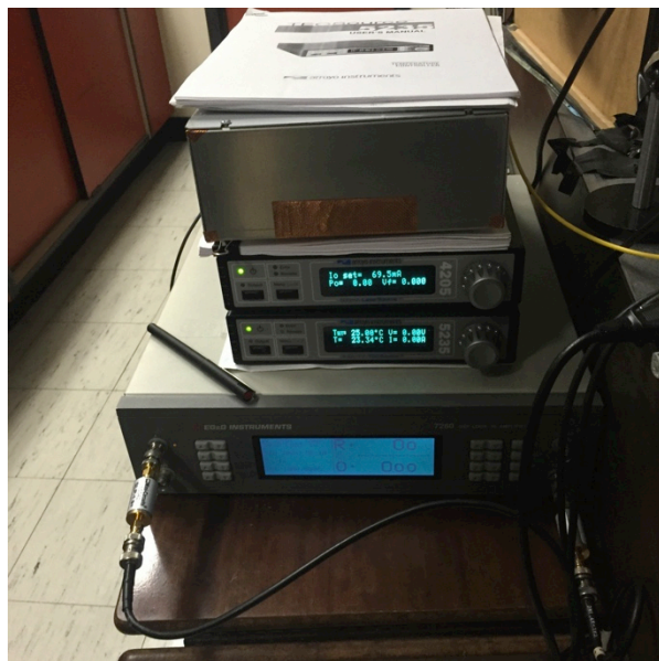
Figure 3. Photograph of electronics for frequency domain measurements showing box containing laser diode and amplifier (top), laser diode current and temperature controllers (middle), and lock-in amplifier (bottom).
