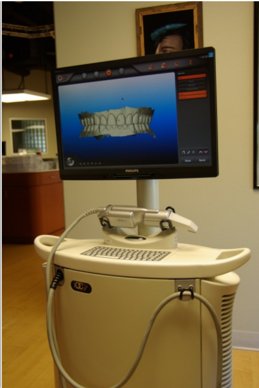
Figure 9. iTero iOC intraoral scanning device.
