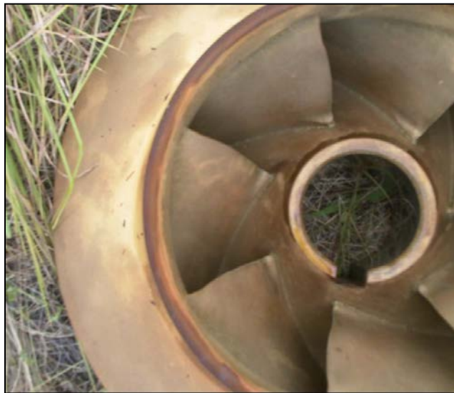
Figure 28. Condition of Unit 2 third-stage impeller after 15 months of exposure, showing minor wear on leading edges.
