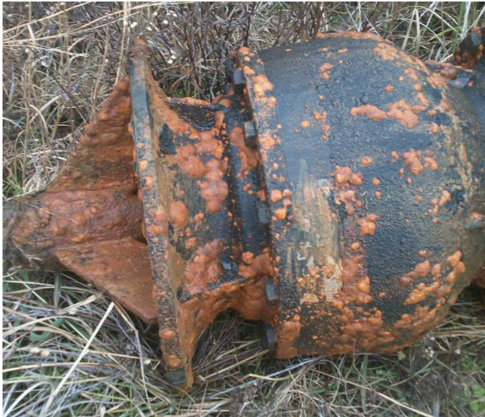
Figure 14. Condition of first state of old Unit 2 pump.
