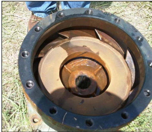
Figure 26. Condition of Unit 1 second stage pump bowl, after 15 months of exposure.
