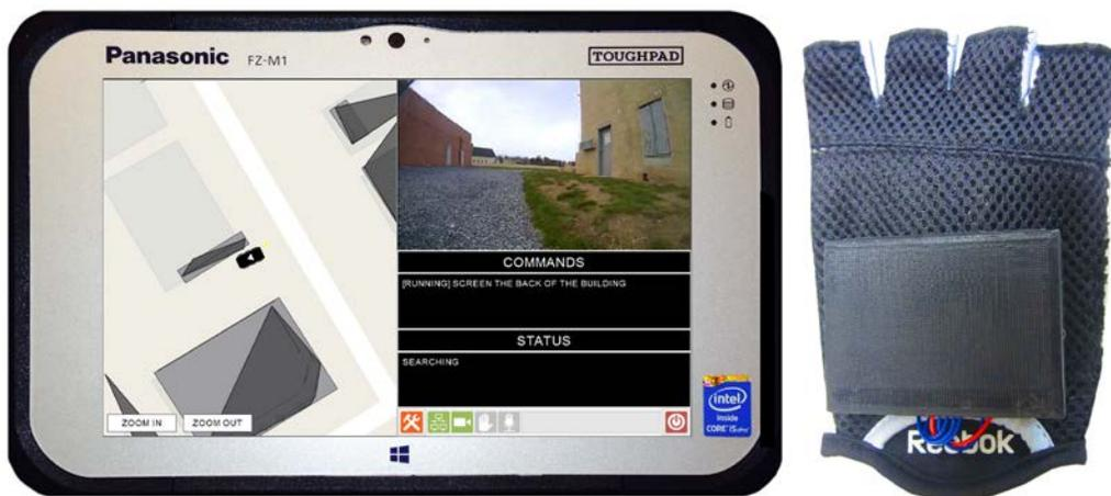
**Fig. 11** The tablet and glove used for and HRI interface. The left side of the tablet’s screen displays a view combining an a priori map from OpenStreetMap (open) with objects in its own world model. The right side, from top to bottom, shows a view through the robot’s camera, the command it is executing, and the activity it is trying to perform.
