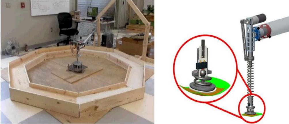
**Fig. 31** (left) The experimental setup for terrain classification using PreSRS on the Hopper. (right) A computer-aided design schematic of the Hopper with PreSRS attached to the bottom of the robot foot.
