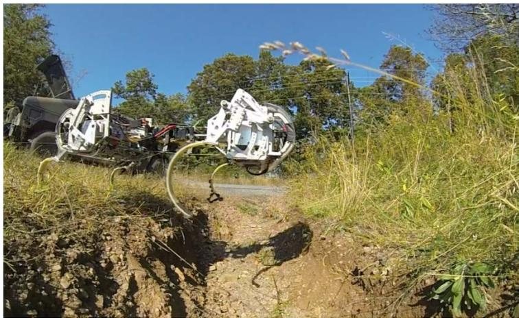
**Fig. 24 Canid leap at drainage ditch**
