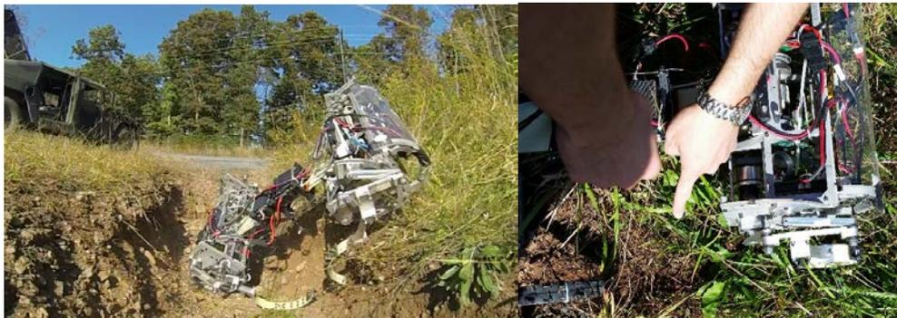
**Fig. 25** Canid after failing to cross the drainage ditch (left) and the ground scuffmarks from insufficient traction in Canid's rear legs while jumping (right)
