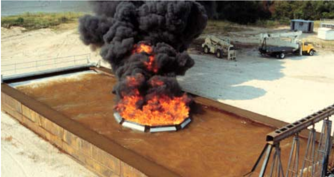
Figure 2. Wave tank (burn pan) with burn in progress.
