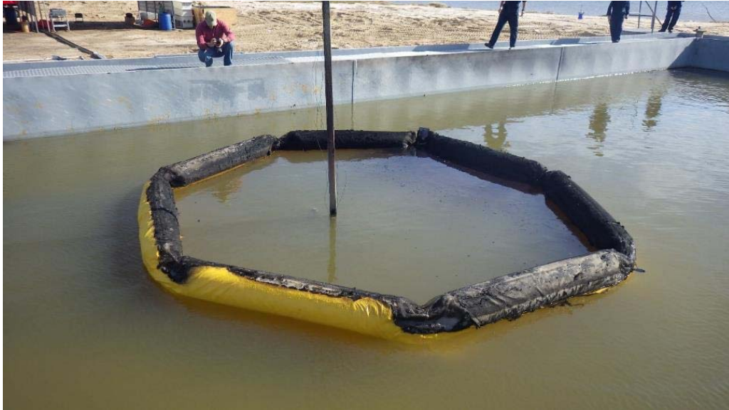
Figure 15. Test 1 - Post-test boom condition.
