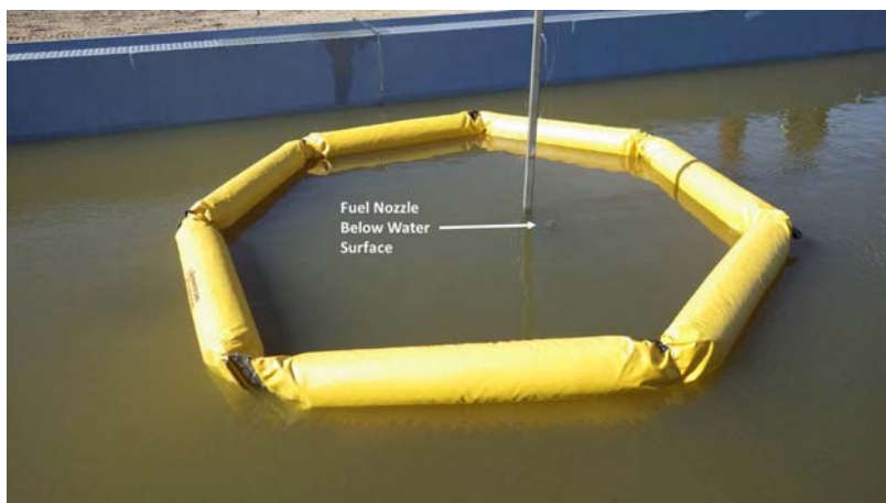
Figure 8. Location of boom with respect to fuel nozzle.
