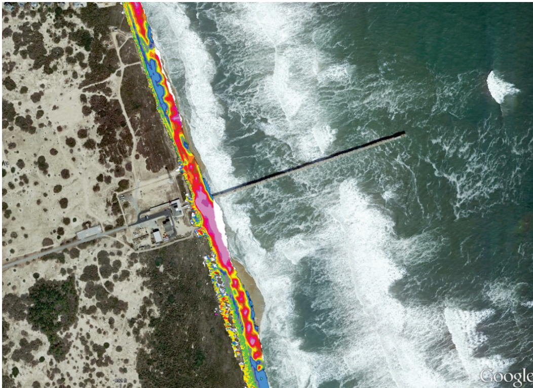
Figure 6. Color-shaded surface elevation difference map between pre- and post-storm dates.
