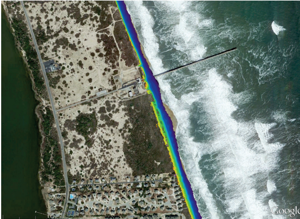
Figure 5. Color-shaded elevation raster displayed over aerial imagery.
