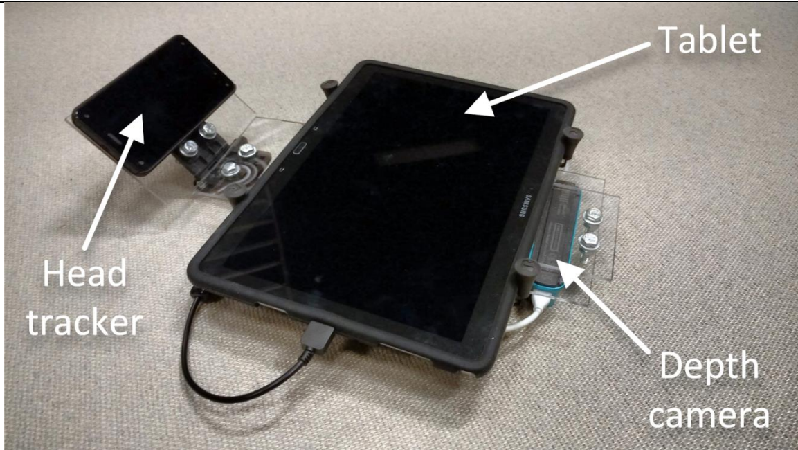
Figure 1: The components of the simulated transparent display used for our analysis.
