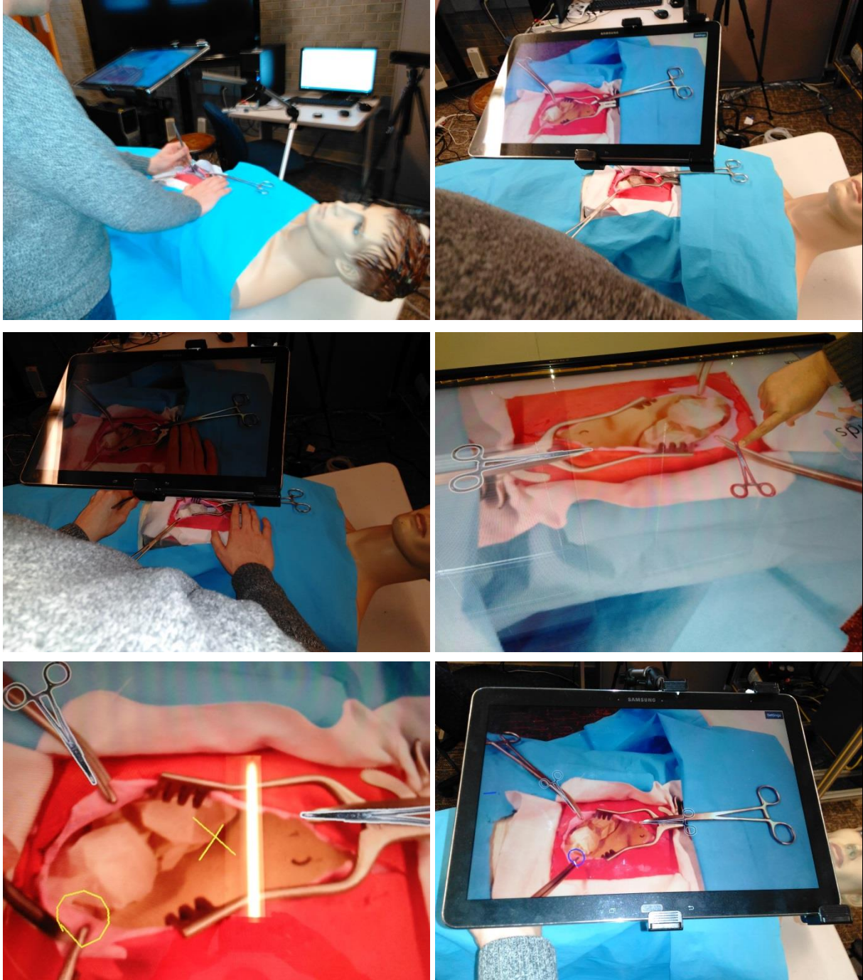
Figure 13. Patient-size Mentor System and Tablet-based Trainee System working together through Wi-Fi
