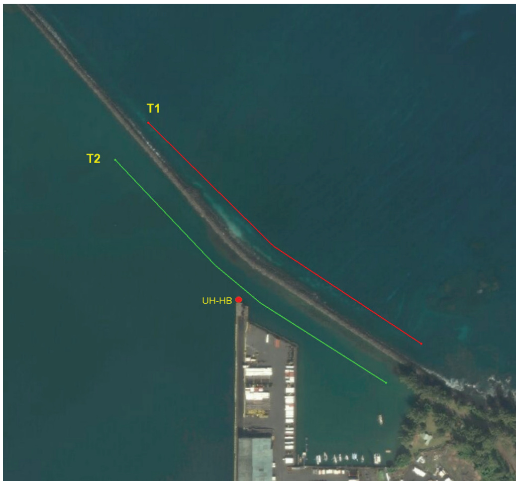
Figure 4-58. Outer and inner transects for breakwater permeability testing.
