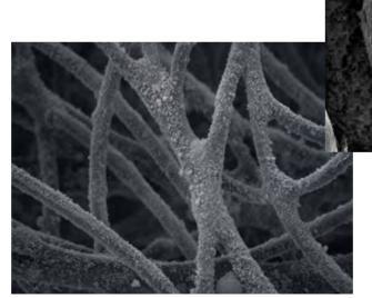
a nanofibrous web surface-coated with a nanoscale adsorbent + catalyst
