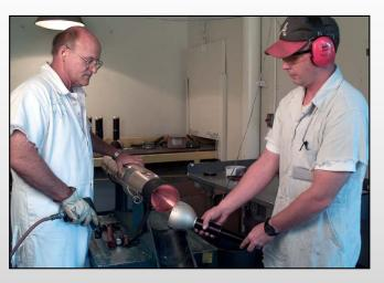
Removal of Crush Switch and Probe from Warhead
