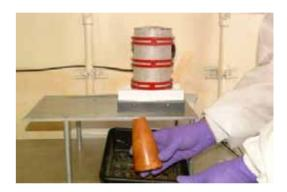
Melted out TNT from 81-MM Mortar
