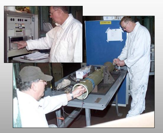
Automated System for Validating Electrical Wiring and Connectors
