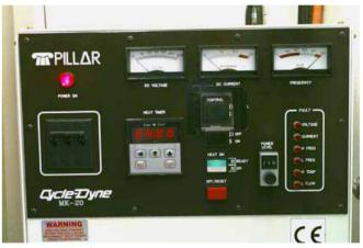
Induction Heating 5kW Power Supply Unit
