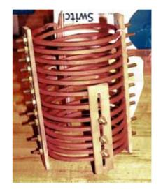
105-mm Projectile Induction Heating Coil
