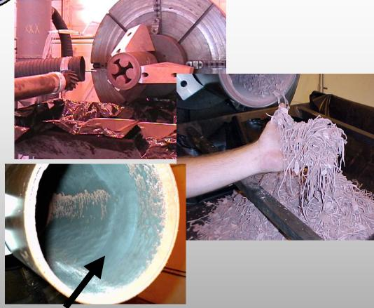
Propellant & liner removed
