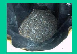
**TOW Rocket Motor & Igniter Grains After Size Reduction**
