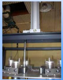
Lift plate holds 6 sonic probe converters.
