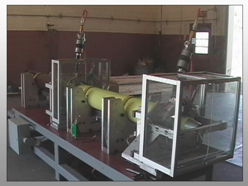
MLRS Warhead/Rocket Motor Separation Station
