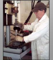
TOW Igniter Assembly Removal Machine
