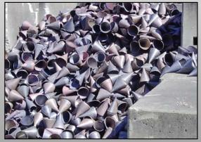
Copper cones after flashing furnace
