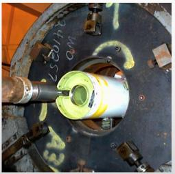
Wire Harness Tube Weldment Removal
