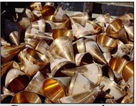
**Copper cones prior to flashing furnace**
