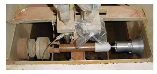
The concept of maintaining the fuse end chuck as an idling component, significantly simplifies the mechanism.
