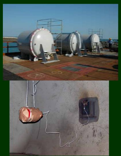
Explosion Experiment Setting, TNT: 2.2kg
