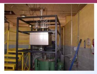
Sonication tank positioned above centrifuge.
