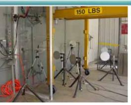
Over-pressure and Thermal Flux Gages
