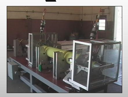
MLRS Warhead/Rocket Motor Separation Station
