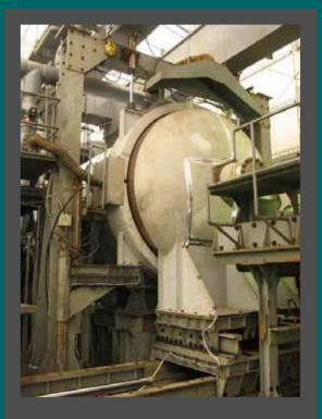
DA VINCH DV60 detonation chamber in Kanda, Japan Destruction of chemical agent and energetic materials in the same time Destruction Mechanism by Implosion
