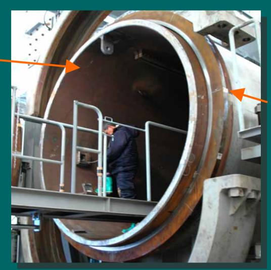
Outer chamber High-pressure vessel against impulsive pressure
