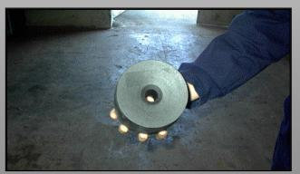
**Recovered TOW Double Base Cartridge-Loaded Grain**
