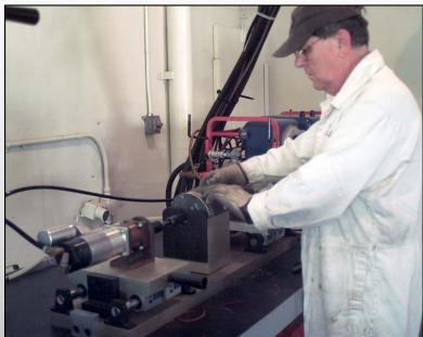
TOW Squib & Retaining Nut Removal Machine
