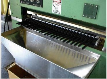
Launch Motor Propellant Shear Machine
