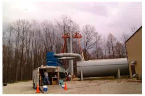
D-200 CDC Stack Test Set-up
