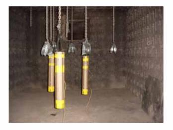
Detonation of Triple 3-in/50 cal cartridges
