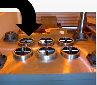
**TOW Grain Splitter Currently Being Fabricated**
