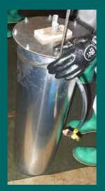
Simulated bomb and emulsion explosive in case\* \*Case made of aluminum for added fireball effect
