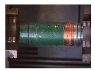
40-mm Projectile after Cutting Operation
