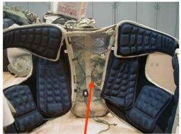
Interior of chassis was unaffected. Slight singeing lower edge of inner pads. 1,000 denier nylon on outside of chassis stayed mostly intact.
