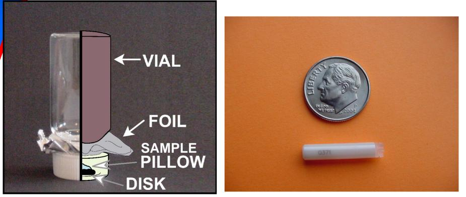
Vapor chamber for exposing catalyst to vaporous agent/simulant Natick Soldier Center, • Natick, MA 4 mm HRMAS rotor for examining small volumes of sample (< 100 μl)
