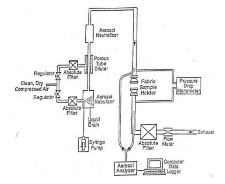
RTI swatch test fixture: aerosol penetration in wind
