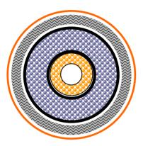
Radial Flow Filter - Inlet flow is directed to outer radial layer first and exits inner core, thus providing significant increase in chemical performance and reduction in airflow resistance
