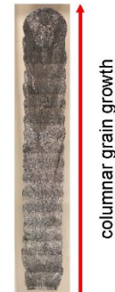
Example Ti-6Al-4V macrostructure from a laser DED build
