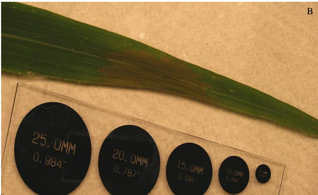
Figure 6. (A) Spread of one 1  $\mu$ L VX droplet, and (B) Target Dot calibration discs and spread of one 3  $\mu$ L VX droplet; each result was photographed on an *E. crus-galli* leaf at 4 h after dissemination of VX onto the foliage.
