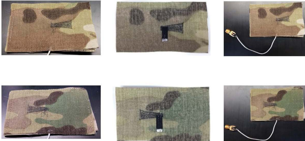
Fig. 11 CNT thread bowtie antenna fabricated on 1,000-denier CORDURA fabric
