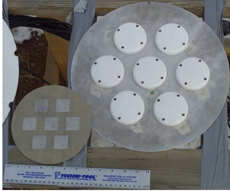
Fig. 6 A basic 7-element CRPA (right) compared with a size-reduced CRPA (left) 13
