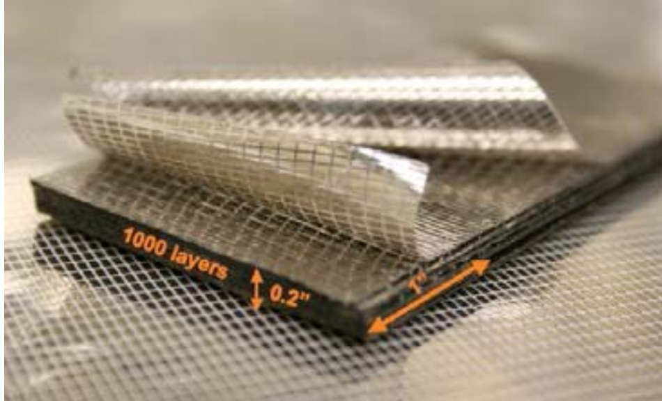
Fig. 16 High-permeability metamaterial substrate using patterned metallic layers
