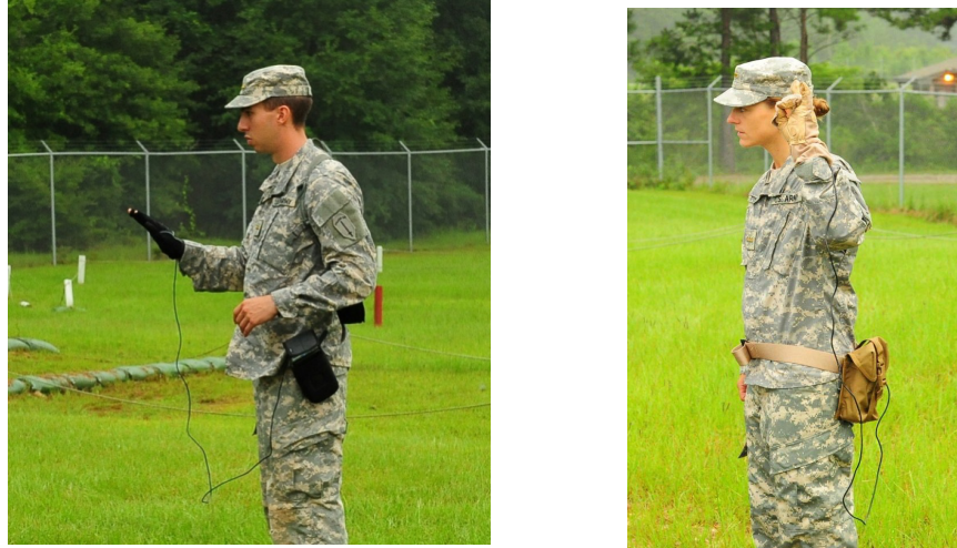
Fig. 2 Soldier using instrumented glove for robot control (left) and communications (right)
