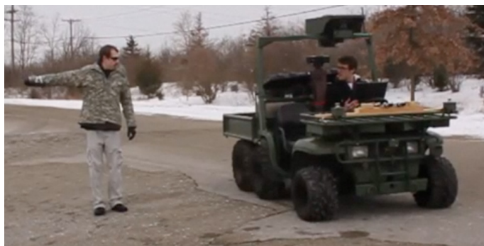
Fig. 1 Camera-based control of robotic mule (Taylor et al. 2012)
