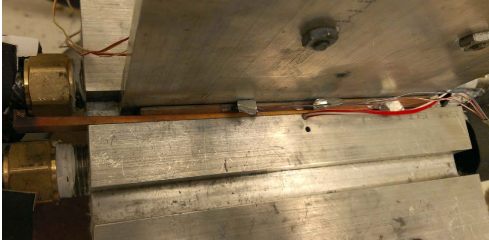
Figure 74: Pulsating-heat-pipe Embedded Design Delivered by MissStateU
