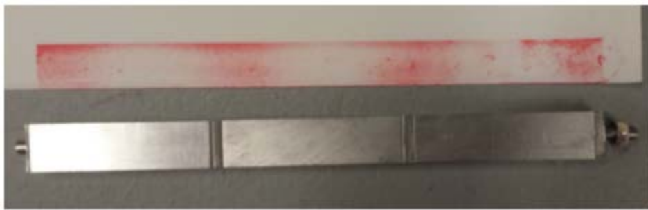
Figure 68: Pressure Distribution for Original Double-sided Wedgelock
