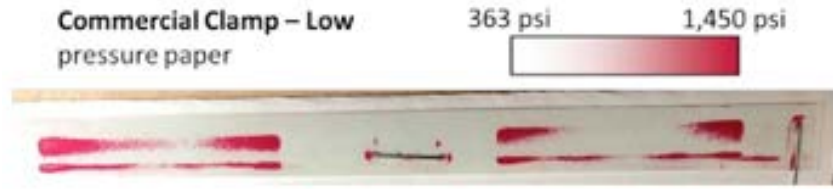
Figure 67: Pressure Paper Tests Results for a Commercial Thermal Connector, Obtained using Low Film
