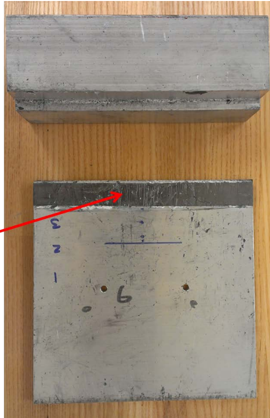
Figure 47: Interface Material Coated on Al Board, Delivered by U of Notre Dame
