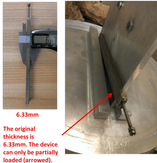
Figure 28: Hydraulic Thermal Connector Delivered by GIT
