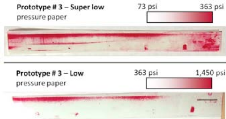
Figure 66: Pressure Paper Tests Results for Prototype # 3, Obtained using Low and Superlow Film
