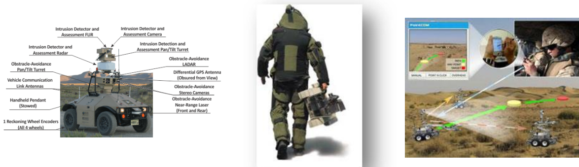
Figure 9-3: Vehicle intelligence involves multiple on-board sensors, autonomy algorithms, and interaction with remote operators and resources.
