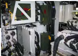
B-Kit components installed into Current Force M1A2 SEP Abrams
