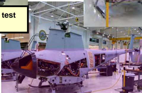
Temporary Nose Cone fitted to Class IV UAV (Fire Scout) A1 preparing for 1 st ever Engine Run at Moss Point Facility (May 07)
