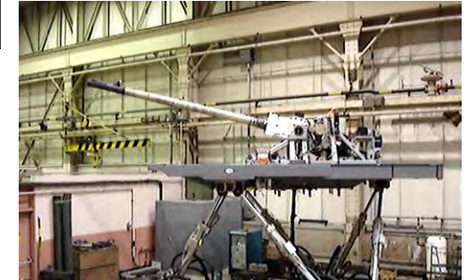
MCS XM360 Electric Gun Elevation Drive Testing
