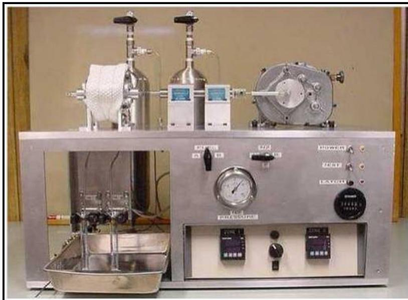
Figure 1. SwRI Dynamic Seal Tester
