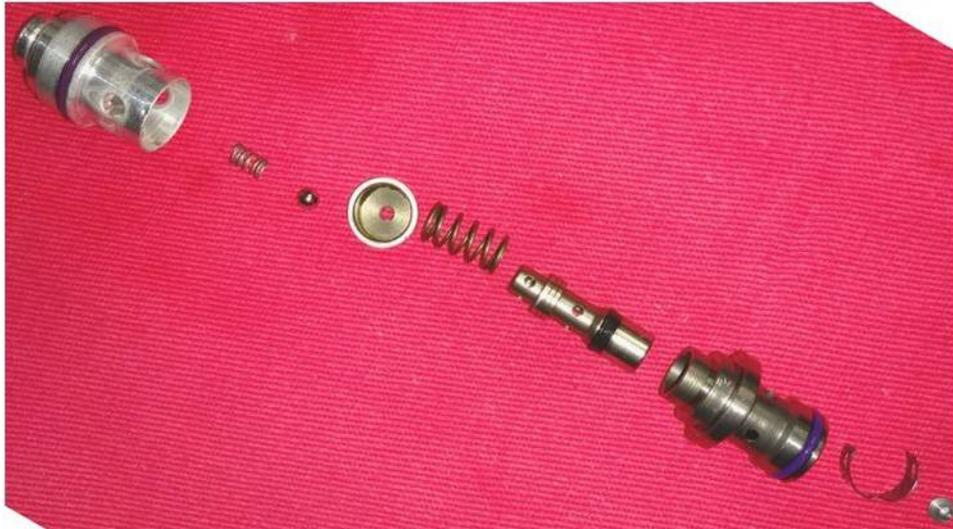
**Figure 23. Disassembled Hydraulic Power Brake Pumping Element**
