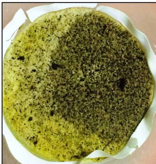
**Figure 19. Filtered Residue from Used HSF**
