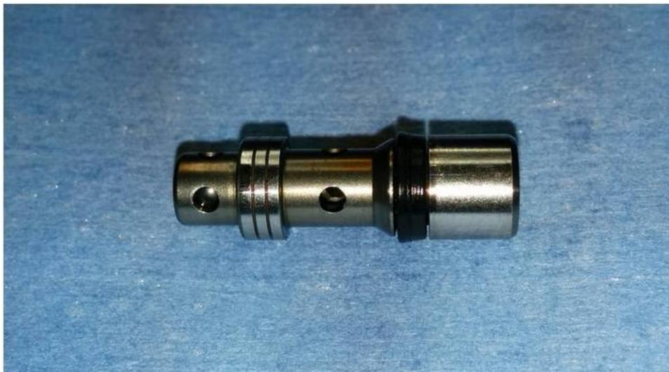
**Figure 24. Hydraulic Power Brake Pumping Plunger Detail**
