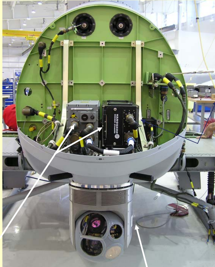
Step Stare Gimbal with MSI Camera
