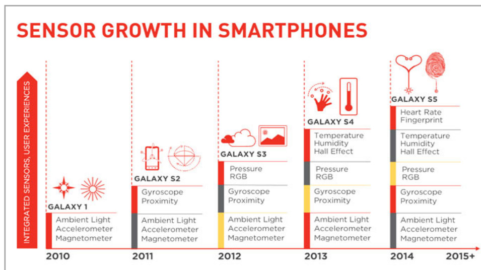
Figure 1. Increasing numbers of sensors added into phones from 2010-2015. [Source: https://www.qualcomm.com/news/snapdragon/2014/04/24/behind-sixth-sense-smartphones-snapdragon-processor-sensor-engine ].
