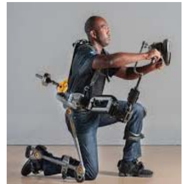
Figure 2. Lockheed Martin Fortis Human Powered Exoskeleton
