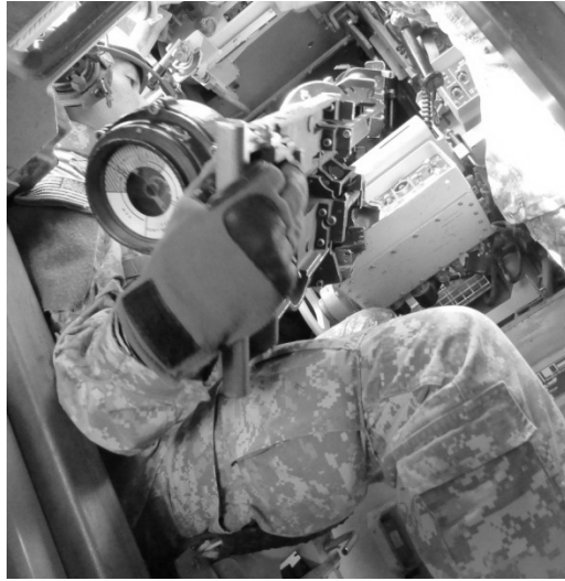
Figure 1.6. Image of Soldier Removing the Feeder Assembly from the 25mm Gun on a BFV (Task 6)
