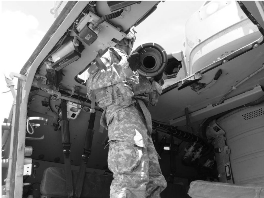
Figure 1.8. Image of Load a TOW Missile Launcher on BFV (Task 8)
