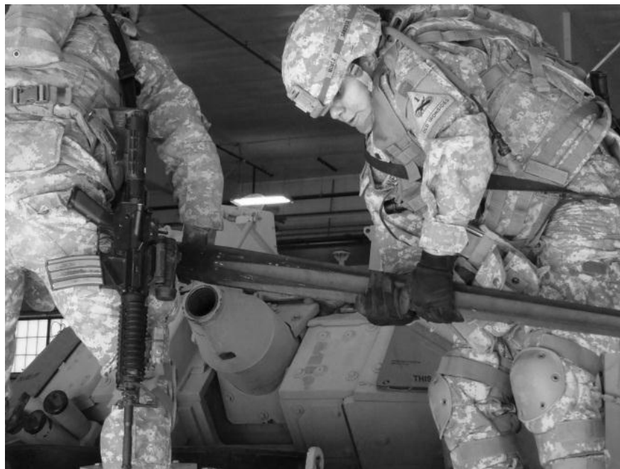
Figure 1.5. Image of Soldier Installing the Barrel of the 25mm Gun on a BFV (Task 5)
