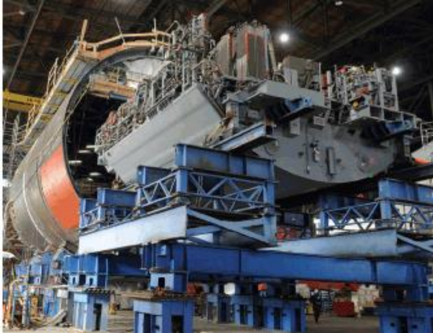
Figure 2. A “raft” being loaded onto USS New Hampshire (SSN 778) at EB’s Quonset Point facility (from Holmander and Plante 2011)
