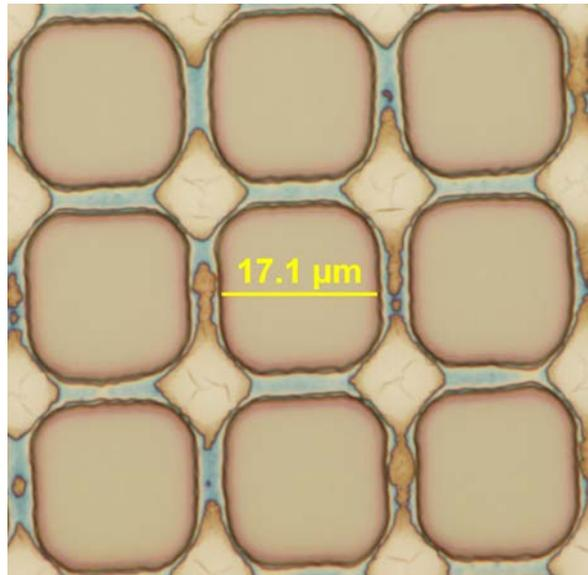
With a slightly longer exposure time, Test Run #2 did not have any connected resonators, but the large print gap created a significant diffraction pattern around the resonator.
