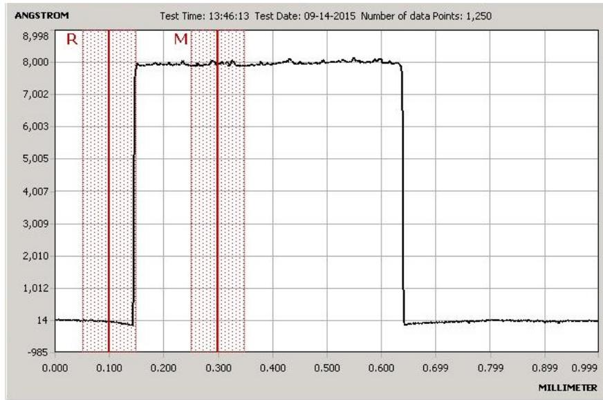
The difference in height between the peak region and baseline region provides the total thickness of aluminum and photoresist over a specified region. Combining this data with the FILMeasure program provides the Al thickness removal for each sputter etch cycle.
