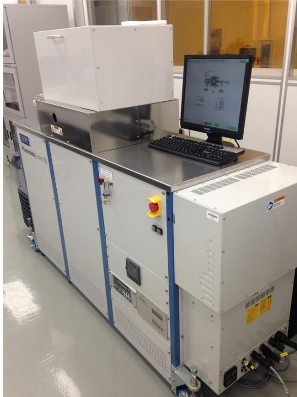
Used for the Ar Sputter Etching of Wafer C-11-34. Two etches, both one minute in duration, were required to remove the requisite amount of aluminum to fabricate the desired metamaterial. Fabrication limitations led to the over etch being approximately 100 nm.
