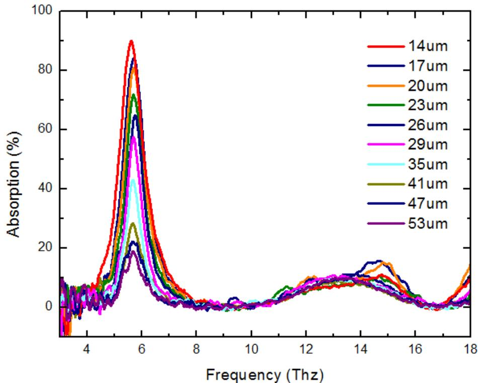
The experimental absorption spectra for wafer C-11-31, with the pitch ranging from 14  $\mu\text{m}$  to 53  $\mu\text{m}$  as denoted in the legend. The square size (12  $\mu\text{m}$ ) was held constant for each region. As the pitch increases, there is a mostly steady decrease in peak absorption, while peak frequency is relatively constant. Although this research is primarily focused on the primary mode between 3-8 THz, note the other modes from 10-18 THz with lower absorption peaks.
