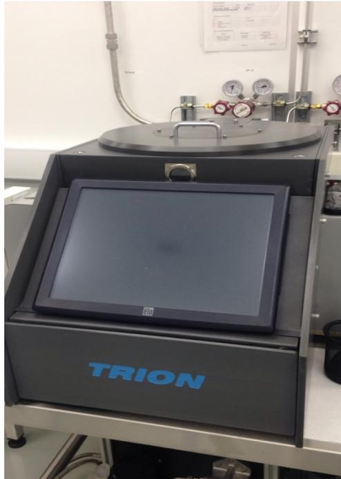
The “Clean” Recipe was used during the final process step in the removal of SPR 955-CM-0.9 photoresist. Conditions were as follows: RF power of 150 W, pressure of 250 millitorr and O<sub>2</sub> flow of 50 standard cubic centimeters per minute.
