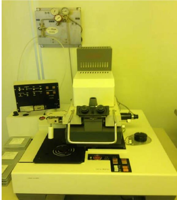
The CMA was used to expose each wafer with UV light during the photolithography process.
