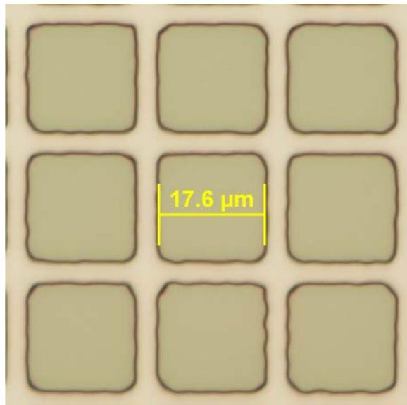
A reduced print gap to 10  $\mu\text{m}$  from 40 $\mu\text{m}$  eliminated diffraction, yet the resonators were clearly distorted and larger than expected. The exact reason for the waviness of the resonator outer edges was not determined, but could have resulted from an unclean mask.
