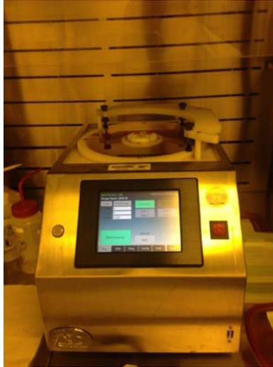
The spin coater distributed the MCC 80/20 Primer and the SPR 955-CM-0.9 Photoresist along the wafer during the pre-lithography phase of fabrication.
