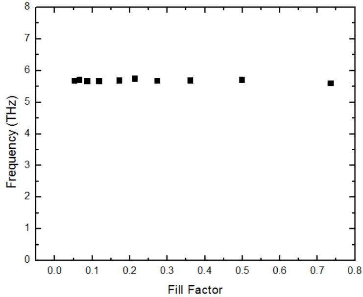
The frequency was relatively constant for C-11-31 as was expected for a resonator with a constant square size.
