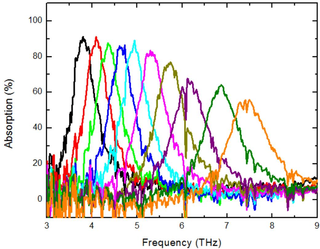
Absorption data for the main mode of C-11-34. Note the shift in peak absorption frequency from the 18  $\mu\text{m}$  square (black curve) to the 9  $\mu\text{m}$  square (orange curve).
