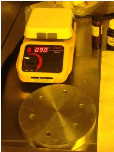
The hot plate was used during the pre-exposure and post exposure bakes. The metal plate (located below the hot plate) let the wafer cool to room temperature immediately after the bakes.
