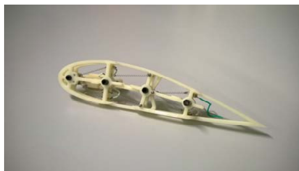
Figure 7 – Articulated wing rib actuated by shape memory springs.
