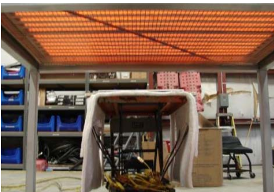
Figure 3. Infrared heater with composite plate test table in position.
