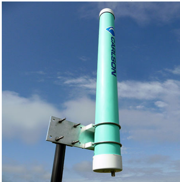
Figure 2.2: Carlson Wireless omni-directional antenna, utilized with base station node
