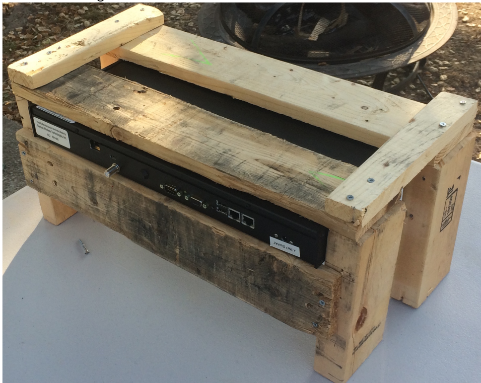
Figure 3.3: Rural Connect TV base station enclosure
