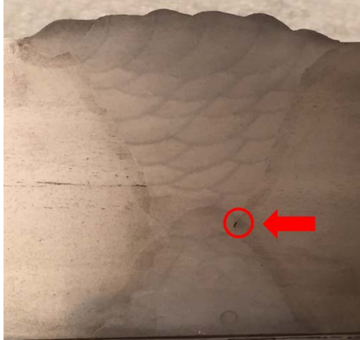
Figure 15. Incomplete Fusion Found in an Experimental B2V.1 70/30 Butt Joint.
