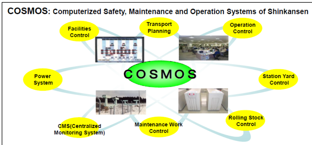
Figure 5. The Integrated Intelligent Transport Management System COSMOS
