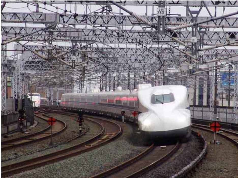
Figure 2. Shinkansen N700-I in Multitrack Urban Setting
