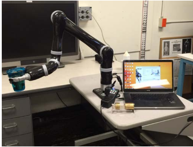
Figure 19. JACO arm to lift weights implementation.
