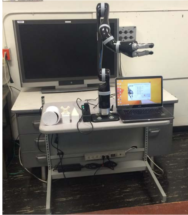
Figure 10. JACO arm with equipment implemented for Joystick trajectory demo.
