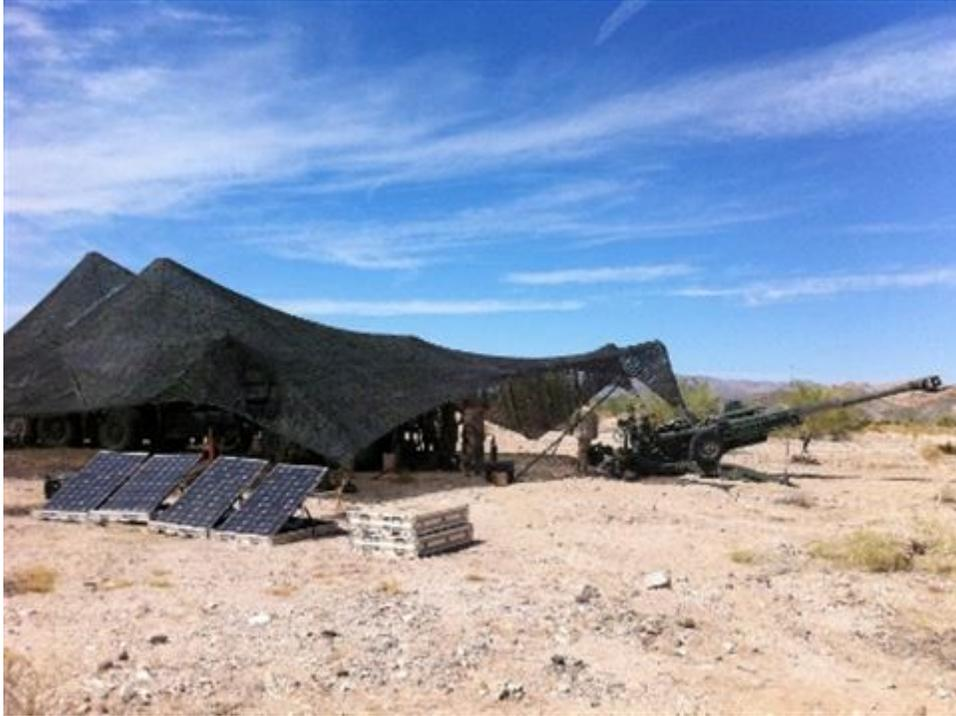
Figure 2. GREENS setup in support of a Marine artillery unit, from [6].
