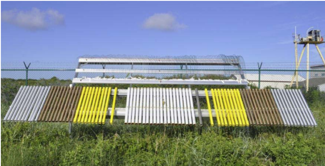
Railing and wire coupons on exposure rack
