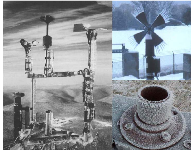
Left and top right: glaze ice on anemometers and wind vanes. Bottom right: hoarfrost that formed under clear night skies.
