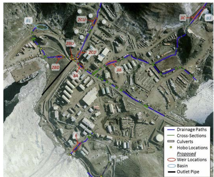
McMurdo Station drainage system.
