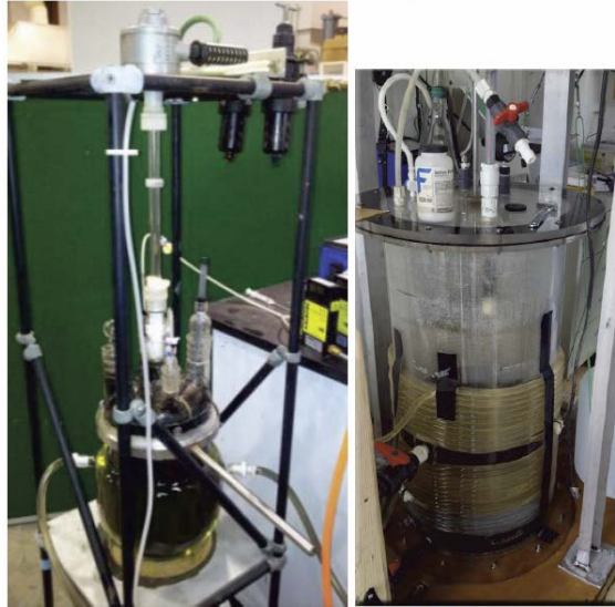
Laboratory and pilot reactors used to study anaerobic digestion for treating Forward Operating Base wastes.
