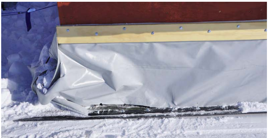
The polymer-coated fabric used for prototype ARCS pouches was stiff to handle at low temperatures and tended to crack when flexed over rough snow.
