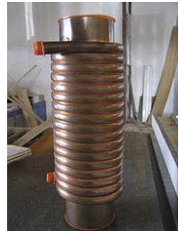
Greywater heat recovery unit
