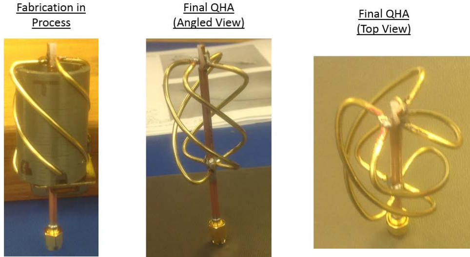
Fig. 24 Fabrication of QHA prototype
