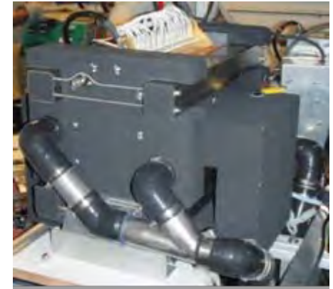
Fuel cell stack with manifolding
