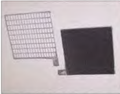
Conventional lead grid (left). Firefly carbon-graphite foam grid (right)
