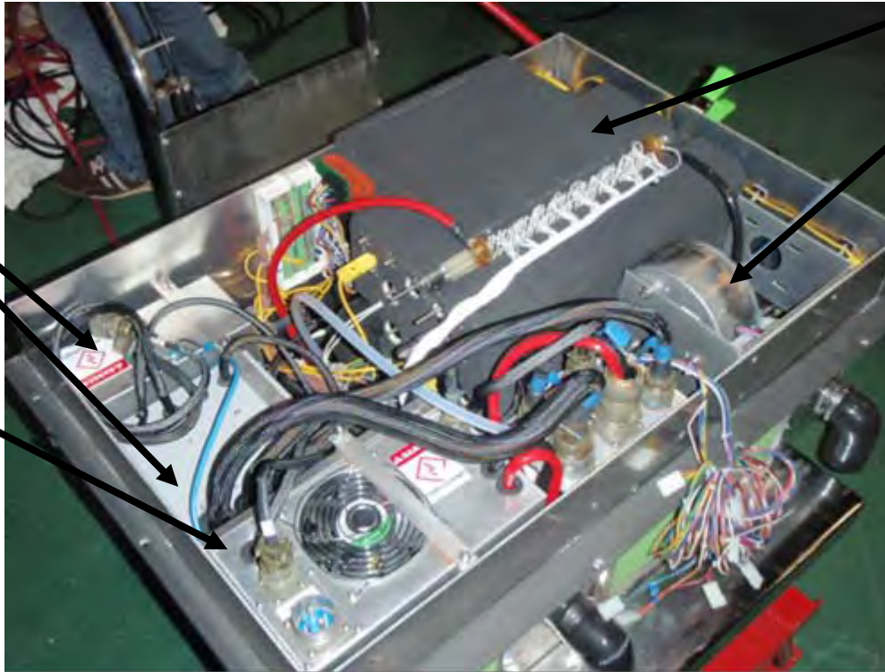
3kWnet TRL-6, HT-PEMFC system prototype
