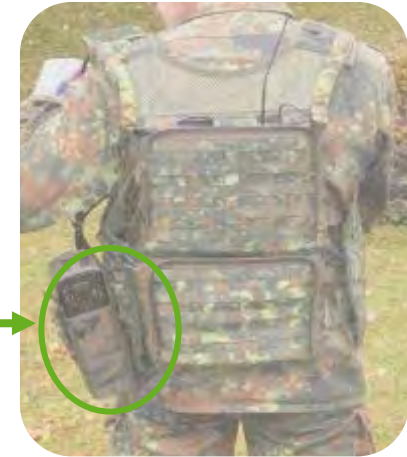
Fuel cell attached to the IdZ system
