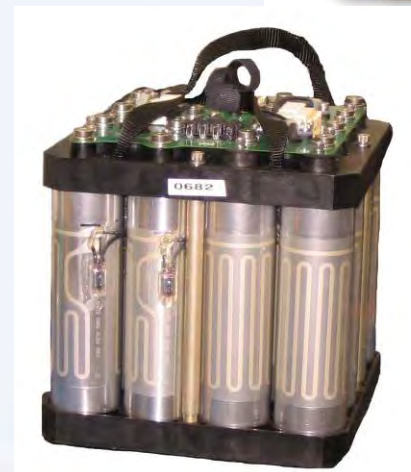
ITAS cell pack: 8S, 2P configuration
